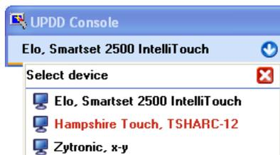
If a USB device is unplugged the name is shown in red in the display area and dropdown. If a serial device is listed in red it indicates either the com port is unavailable to the driver or that the initialisation macro (if one exists for the device) has failed. Depending on the type of macro failure the device could still be operational. The Calibration option is disabled on devices deemed unavailable.
